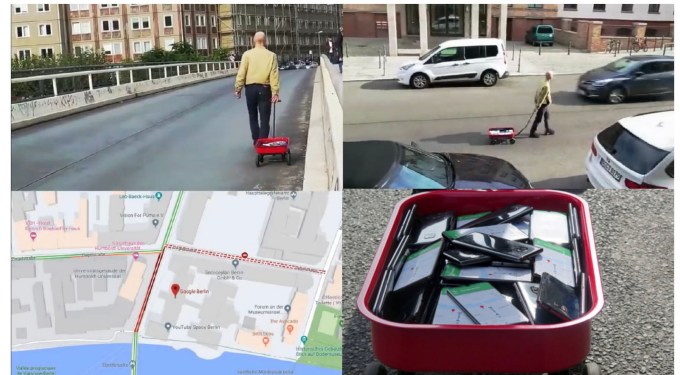
Fig. 12. A case of cheating existing monitoring Apps with a small toy trailer of mobile phones: Google map shows that the street is heavily congested while the traffic of the street is quite smooth [44].
