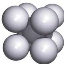
$$\begin{aligned} r &= a\sqrt{3}/4; \text{ also } Z = 2 \therefore D = \frac{\text{sphere volume}}{\frac{1}{2}(\text{unit cell volume})} \\ &= \frac{1.33\pi r^3}{0.5a^3} = \frac{1.33\pi r^3}{0.5\left(\frac{4r}{\sqrt{3}}\right)^3} = 0.6802 \end{aligned}$$
