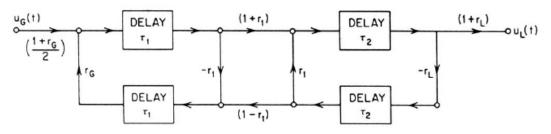
Fig. 3.37 Complete flow diagram of a two-tube model.
