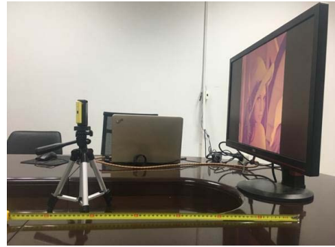
Fig. 13. The experimental sketch of the recapture process.
