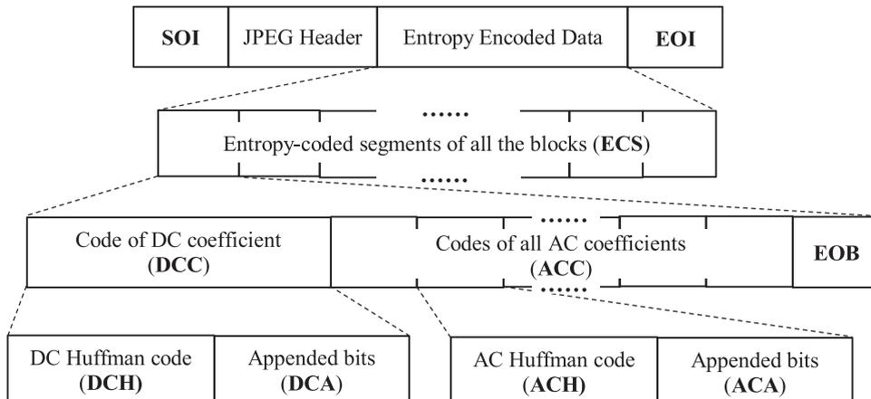
Fig. 4. Simplified syntax of JPEG baseline. SOI, EOI and EOB stand for start-of-image, end-of-image and end-of-block respectively. Acronyms in the parentheses are used in the discussion for brevity.
