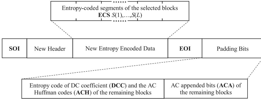
Fig. 5. Syntax of the new JPEG bitstream.
