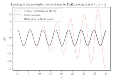
Here the differences between  $\mathcal{O}(\varepsilon)$  approaches for both regular perturbation theory and multiple-scale analysis can be seen, and how they compare to the exact solution for  $\varepsilon = \frac{1}{4}$
