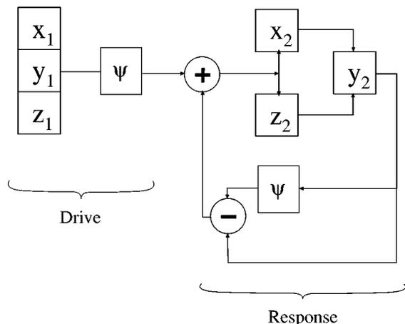
FIG. 10. Schematic for synchronous substitution using a filter.
