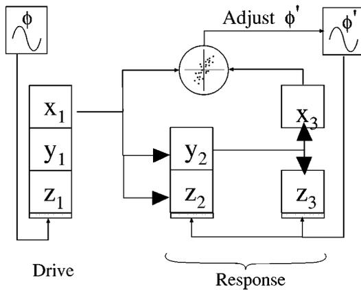
FIG. 9. Nonautonomous synchronization schematic. The local periodic drive is indicated as going into the “bottom” of the drive or response, but it can show up in any or all blocks. The incoming signal  $x_1$  is compared to the outgoing  $x_3$  using a strobe. When the periodic drives are out of phase (i.e.,  $\phi \neq \phi'$ ) we will see a pattern in the strobe  $x_1-x_3$  diagram that will allow us to adjust  $\phi'$  to match  $\phi$ .
