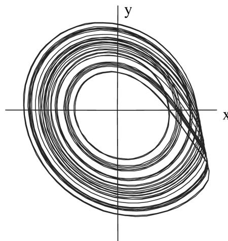
FIG. 16. The circuit Rössler attractor.
