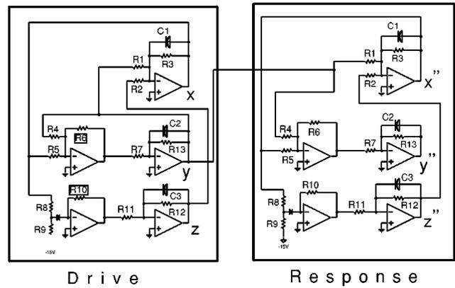
FIG. 6. Piecewise linear Rössler circuits arranged for cascaded synchronization.  $R1=100\text{ k}\Omega$ ,  $R2=200\text{ k}\Omega$ ,  $R3=R13=2\text{ M}\Omega$ ,  $R4=75\text{ k}\Omega$ ,  $R5=10\text{ k}\Omega$ ,  $R6=10\text{ k}\Omega$ ,  $R7=100\text{ k}\Omega$ ,  $R8=10\text{ k}\Omega$ ,  $R9=68\text{ k}\Omega$ ,  $R10=150\text{ k}\Omega$ ,  $R11=100\text{ k}\Omega$ ,  $R12=100\text{ k}\Omega$ ,  $C1=C2=C3=0.001\text{ }\mu\text{F}$ , and the diode is a type MV2101.
