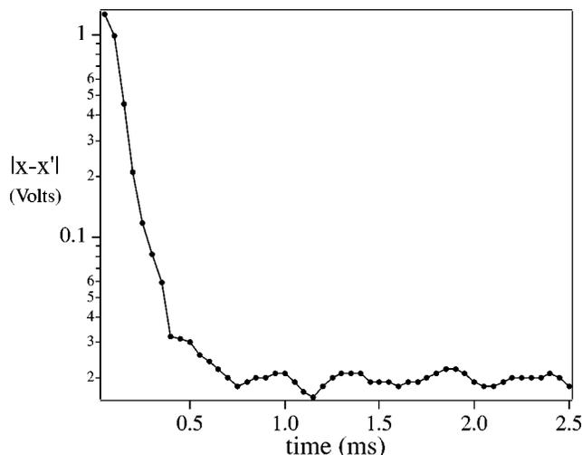
FIG. 12. The BK method is demonstrated on the piecewise-linear Rössler circuit. The difference in the  $X$  variables of receiver and transmitter is shown to converge to about 20 mV in under one cycle of the period-1 orbit (about 1 ms). The plot is an average of 100 trials.
