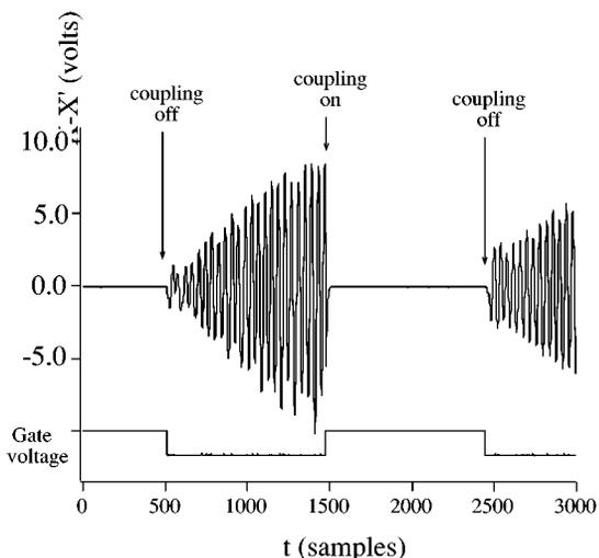
FIG. 14. The BK method as applied to the hyperchaotic circuit. The coupling is switched on when the pictured gate voltage is high, and **B** is effectively  $\{0,0,0,0\}$  when the gate voltage is low. The sample rate is  $20 \mu\text{s}/\text{sample}$ .
