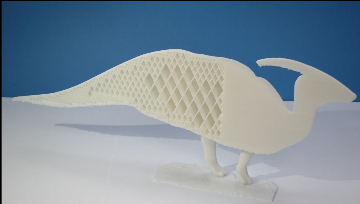
The printed cross section of the Dilo model [Wu et al. 2016]
