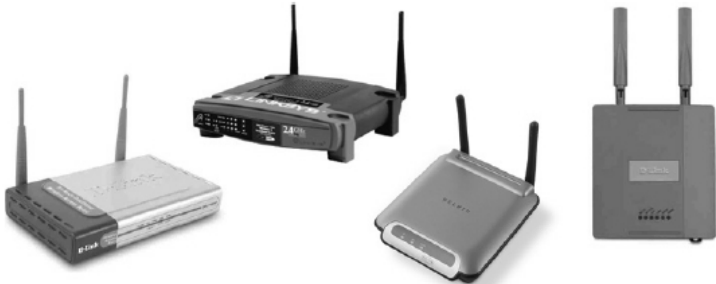
Figure 3-10: First Generation Wireless Access Points (courtesy of Belkin Corporation, D-Link (Europe) Ltd. and Linksys (a division of Cisco Systems Inc.))
