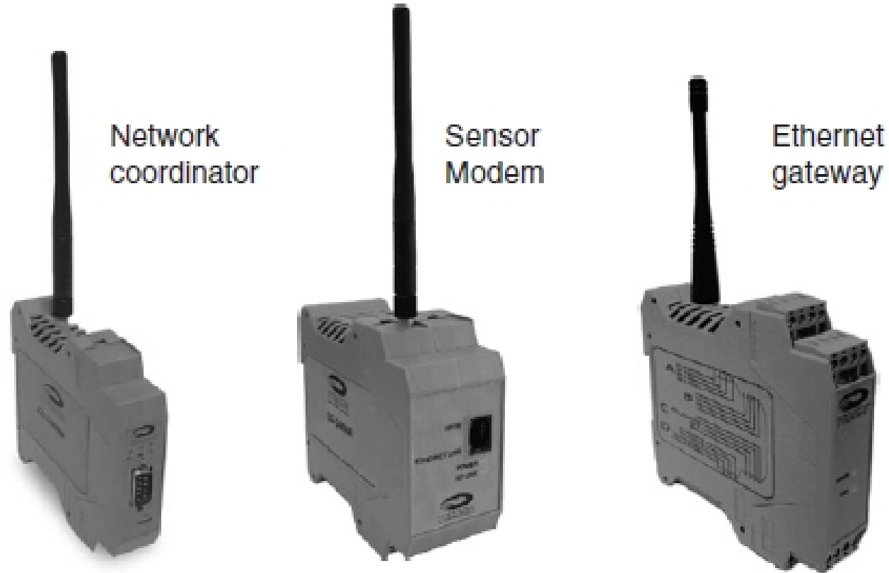
Figure 3-21: A Variety of ZigBee Devices (courtesy of Cirronet Inc.)
