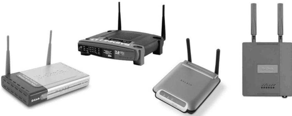
**Figure 3-10: First Generation Wireless Access Points** (courtesy of Belkin Corporation, D-Link (Europe) Ltd. and Linksys (a division of Cisco Systems Inc.))
