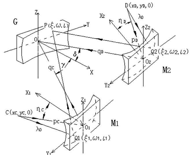
Fig. 5. Schematic diagram of recording holographic grating.
