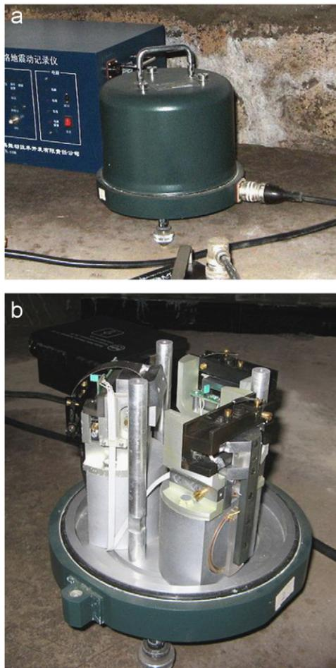
Fig. 16. Triaxial velocity sensor for the JC-V104 digital seismograph: (a) outside view; (b) internal components.
