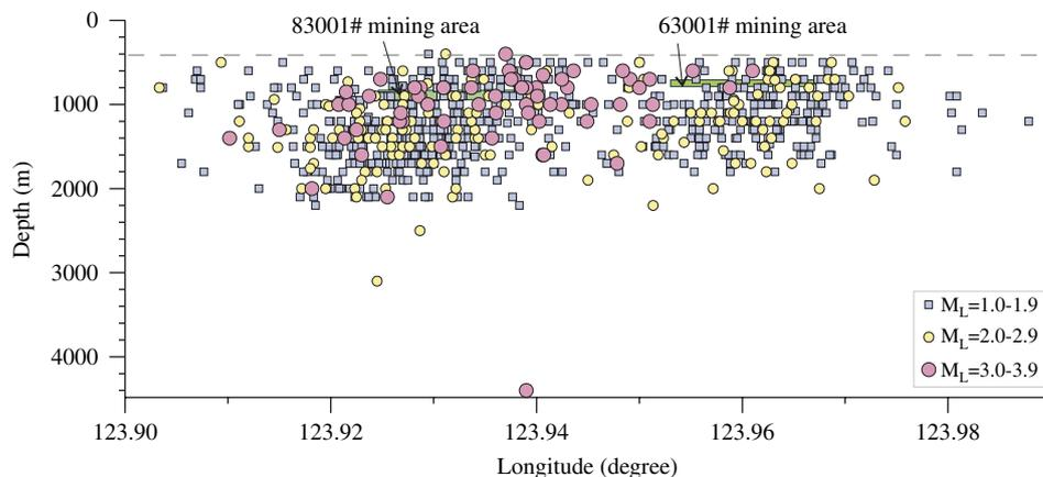
Fig. 4. Seismic event source location distribution (from July, 2003 to June, 2004) at Laohutai coalmine, Fushun, Liaoning Province.
