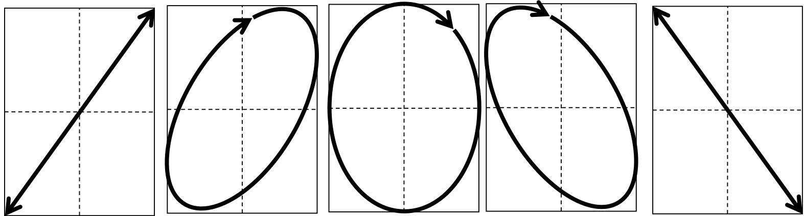
$$\Delta\varphi = \pi \quad \Delta\varphi \in (\pi, \frac{3\pi}{2}) \quad \Delta\varphi = \frac{3\pi}{2} \quad \Delta\varphi \in (\frac{3\pi}{2}, 2\pi) \quad \Delta\varphi = 2\pi$$
