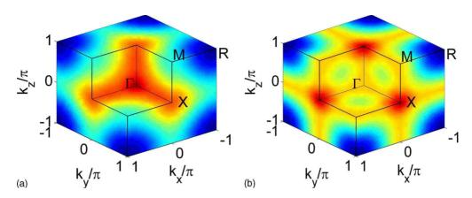
FIG. 9. (Color online) Three-dimensional energy spectrum of the surface states for the parameters (a) c=1, m=-3 and (b) c=1, m=-1. The Dirac points where energy gap vanishes are marked with deepest red color. For m=-3 there is one Dirac point at  $\Gamma$  point, while for m=-1 there are three of them at X points.
