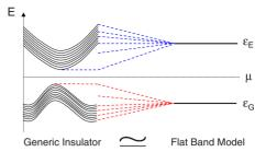
FIG. 8. (Color online) Illustration showing that a band insulator with arbitrary band structure  $\varepsilon_i(k)$  can be continuously deformed to a flat band model with the same eigenstates. Since no level crossing occurs at the Fermi level, the two Hamiltonians are topologically equivalent.
