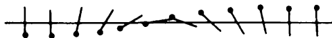
Fig. 10.3. Pegs on a line representing the kink (soliton) solution to the sine-Gordon equation.
