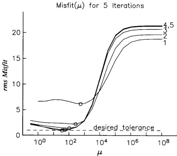
FIG. 3. The rms misfit as a function of the Lagrange multiplier  $\mu$  at five iterations of an inversion. The values of  $\mu$  and misfit chosen for each iteration are marked by symbols and also given in Table 1. The corresponding intermediate models are shown in Figure 4.
